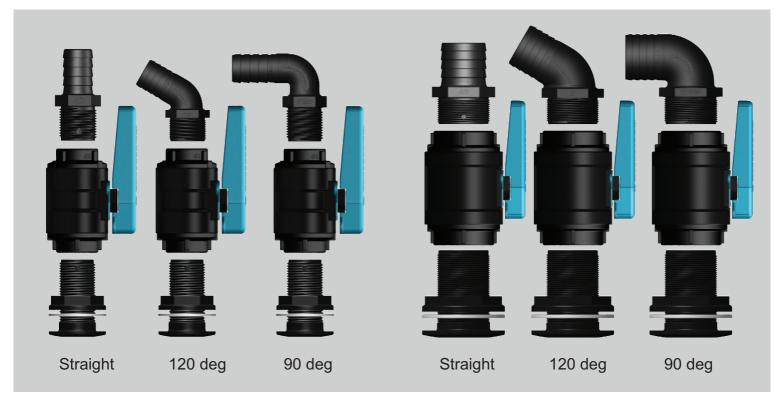
**Tru-Design** range of Skin Fittings are the first composite through hull fitting to be certified by the International Marine Certification Institute (IMCI) Belgium. Designed and made in New Zealand, the Skin Fitting body and nut are moulded from glass fibre reinforced nylon composite. High strength, high-modulus glass fibres provide dramatic strength, stiffness, toughness and dimensional stability.
