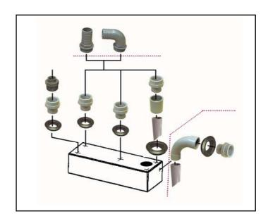
11. Install hose tails using suitable sealant or PTFE tape. Note the ability to rotate the fittings in the Uniseal to allow for correct alignment, particularly helpful when fitting 90° elbows..
