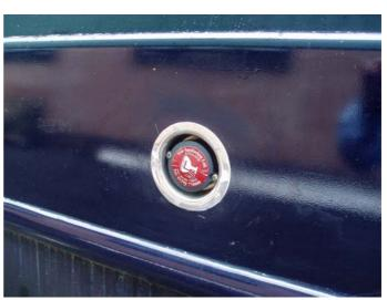
6. Identify position of Tank Level Indicator. This should NOT be too close to the inlet as incoming waste will cause unit to give false readings.
