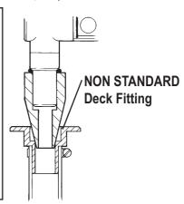
Efficient Pump-Out depends on a good Vaccum (good seal) LEESAN ISO Std. equipment uses "O" Rings to create the "optimum" seal! Where Non Standard deck fittings have been installed, **LEESAN** adaptors are available
