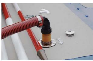
Having emptied the tank, disconnect the pipe from the deck fitting and rinse the unit through with pumping raw water
