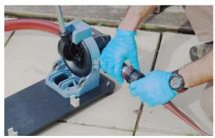
Rinse the pump and pipework with Raw water to check the connection and pump
