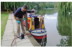
Open the Deck fitting on the boat and connect the suction pipe
