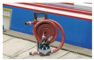
Lay the hose out to the Elsan disposal point and make the connection to the pump
