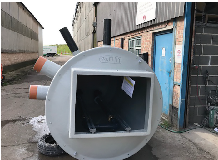
A highly unusual four-pump system with large incoming inlet connection. Just another example of the bespoke jobs the Pegasus team manufacture in-house.
