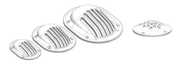
The Scoop Strainer is designed to divert large objects away from water intakes while the vessel is moving. This helps eliminate problems with seaweed/seagrass, sticks or rubbish being sucked into engine intakes and blocking or clogging intake filters. The strainer acts as a course first stage filter that is cleaned by water movement.
